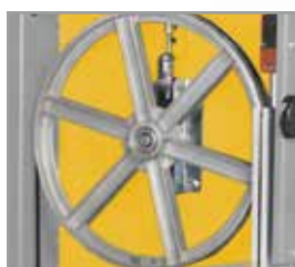
354mm flywheels and blade tensioning device
