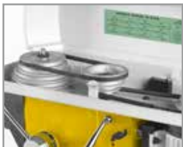
Upper cover opening with safety microswitch
