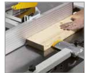
Aluminium parallel guide for upper table works
