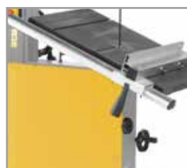
Maximum cutting height up to 224 mm
