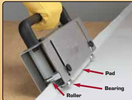
Use repetitive motions to gently bend edge upward. Rollers at the ends of stops and a plastic pad at base of tool assure smooth, non-marring operation.
