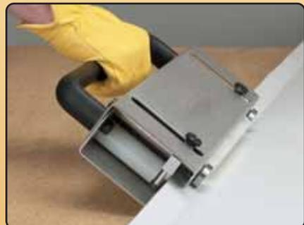
Slide tool over edge of metal and make a score by gliding tool along full length of panel.
