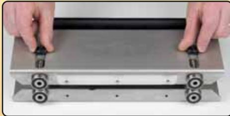
Set the bending depth. Easy-to-adjust thumbscrews quickly lock in the stop gauges without the use of tools.
